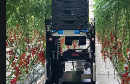
Crates are set at fixed position using sensor and conveyor
