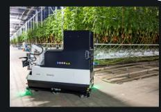
Can drive automatically from lane to lane. Sensor detects obstacles and Pipe rail
