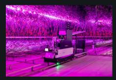
Can drive to a point to discharge the filled crates and put new crates on the robot
