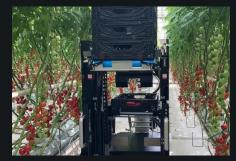
Crates are set at fixed position using sensor and conveyer
