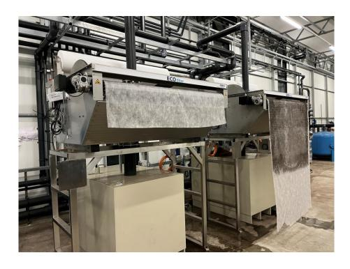
Before treating the water with ozone all particles, wich float in the water, has to be removed. This can also be achieved without water loss
